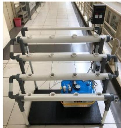
Gambar 4. Foto Setup Sistem Kontrol Nutrisi Berbasis Monitoring IoT
