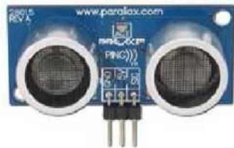
**Gambar 2.12 Sensor jarak ultrasonik ping**
